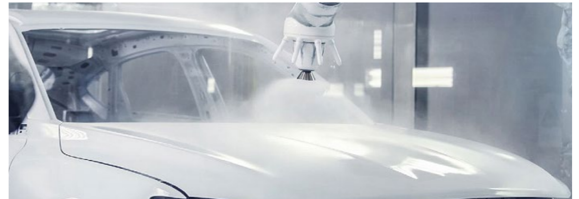
Geely Auto's Xi'an plant uses a fully automated spraying process to reduce energy consumption.
